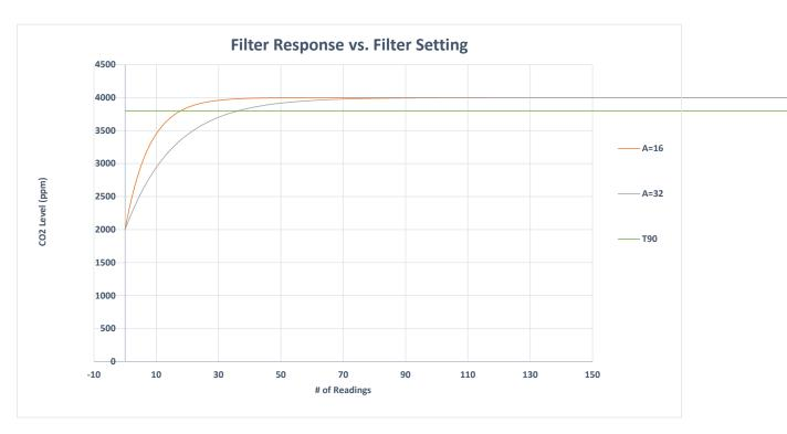
The graph above shows the effect of the filter on response times. Increasing the filter setting increases the measurement output response time.  $T_{90}$  is the time to 90% of reading. The CozIR®-LP3 takes 2 readings per second. The CozIR®-LP3 sensor will also output the raw unfiltered CO<sub>2</sub> measurement data. This data can be post processed using alternative filter algorithms.
